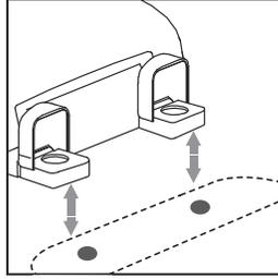
Lift seat up to remove seat from posts.
